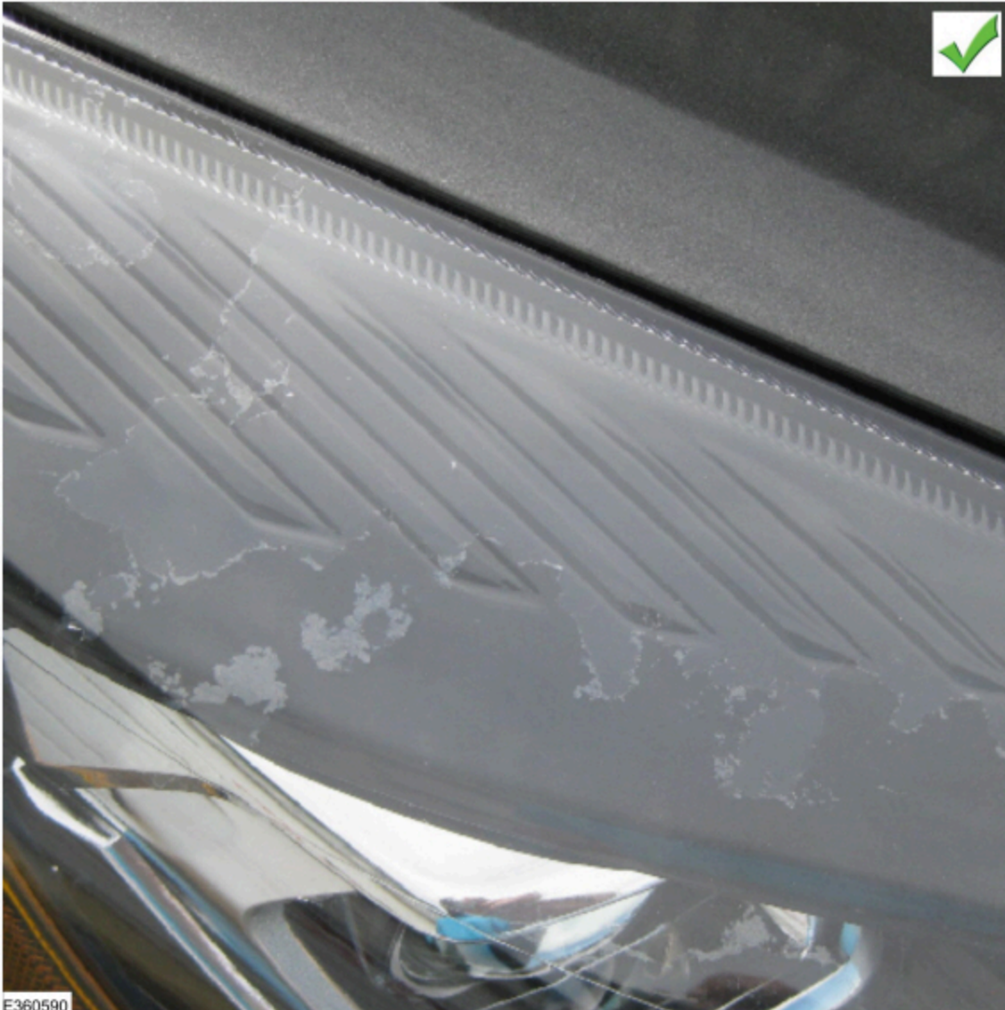
Figure 14 - example of "crazing" - warrantable
