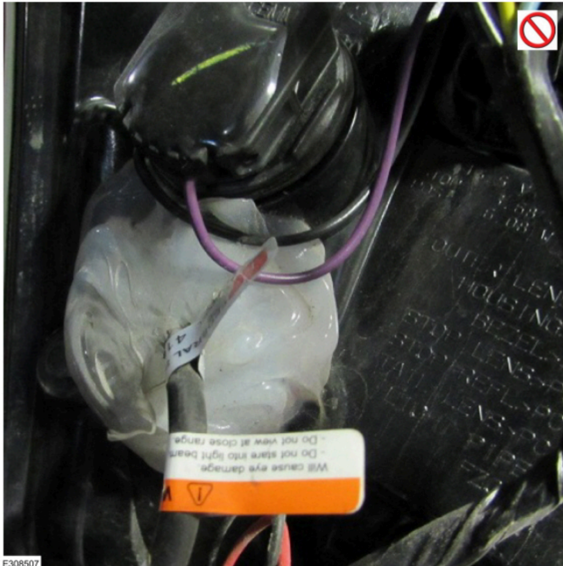
Figure 11 - example of external impact damage - not covered under warranty
