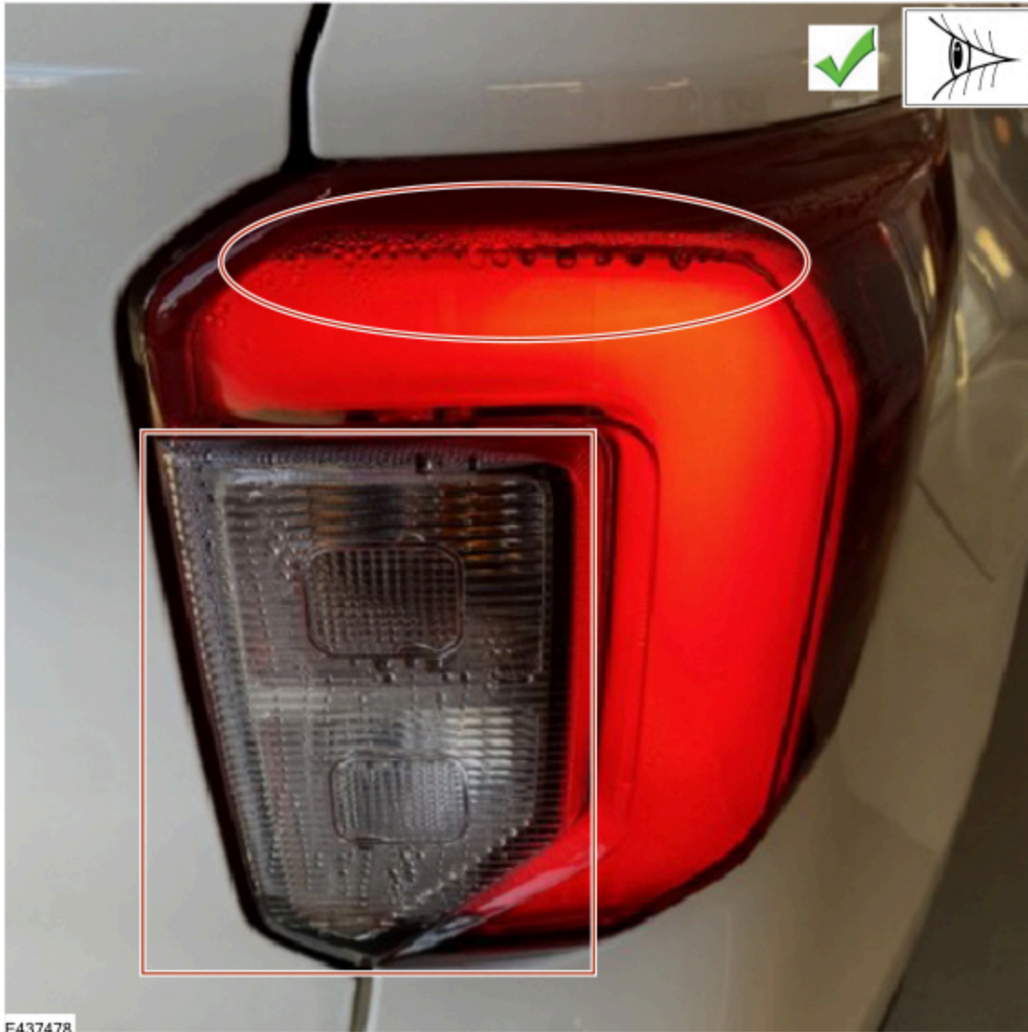
Figure 7 - example of water leak (streaking) - warrantable
