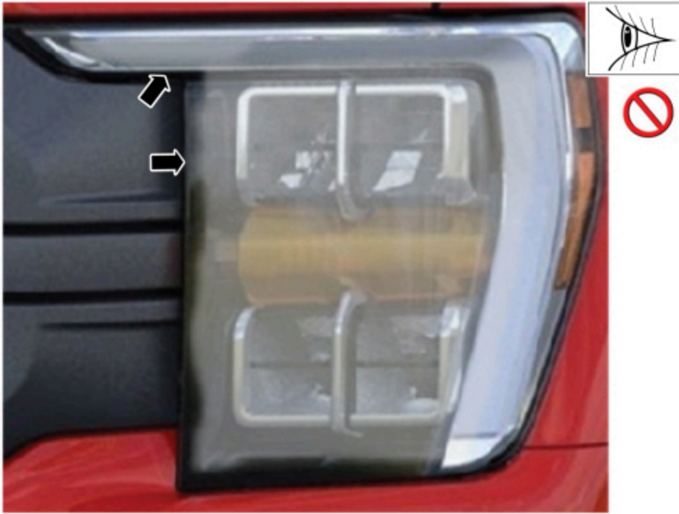
Figure 6 - example of water leak (large droplets) - warrantable
