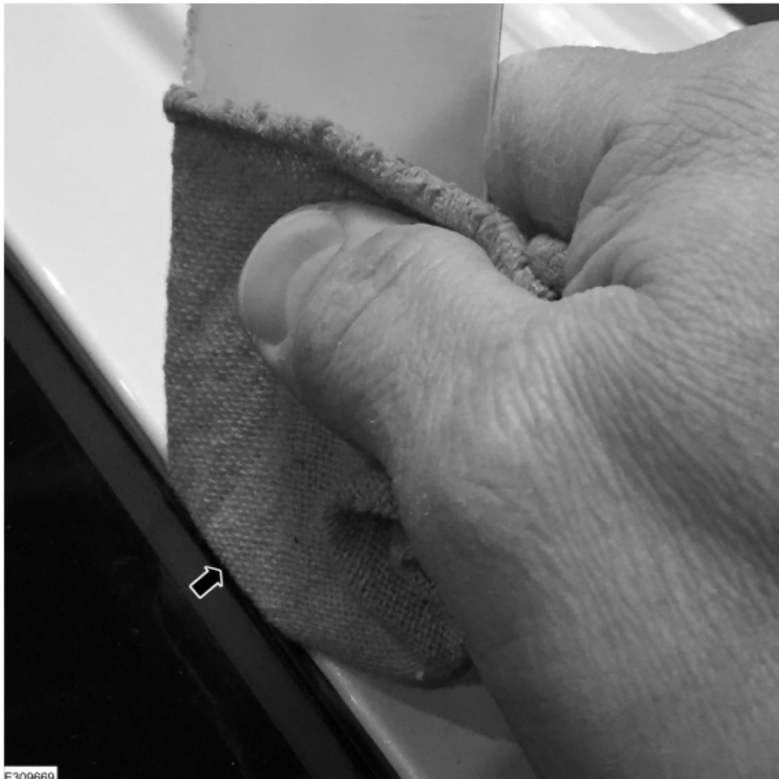
8. Apply a light film of Krytox® grease to the entire sheet metal roof opening of the movable glass panel and the front edge of the movable glass seal.
