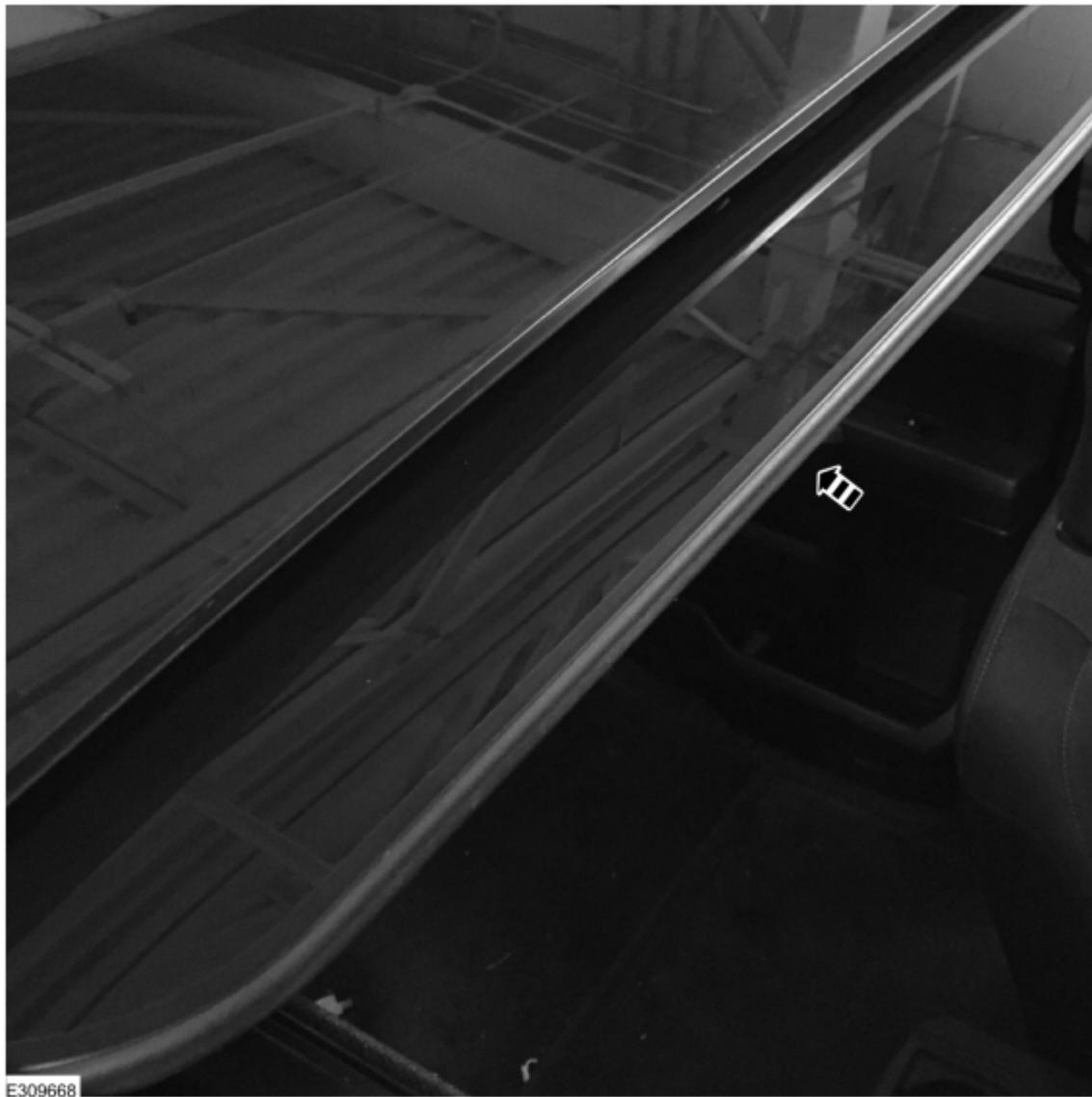
5. Clean the remaining front rubber seal area of the movable glass panel with isopropyl alcohol or equivalent.
