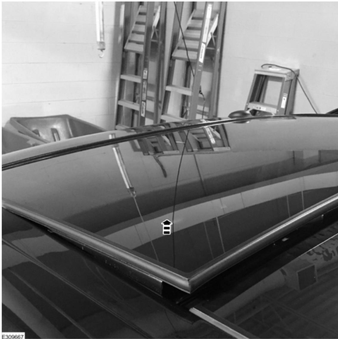
2. Clean the rear and side rubber seals of the movable glass panel with isopropyl alcohol or equivalent.
