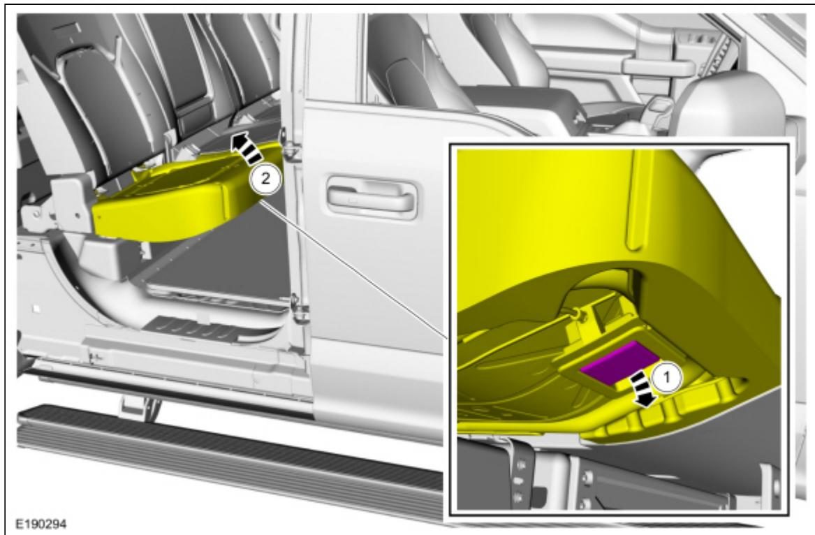
13. Release the taps, clips and position aside the cover.
