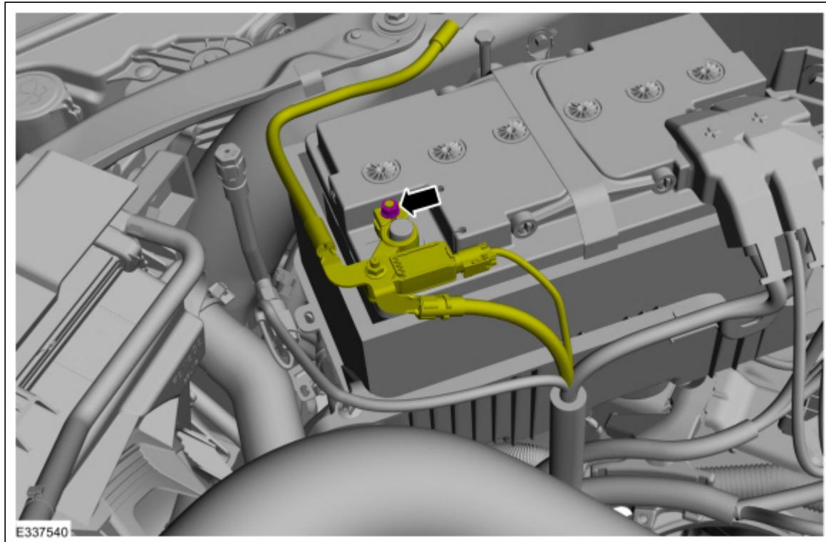
2. Position the positive battery cable terminal cover aside.
