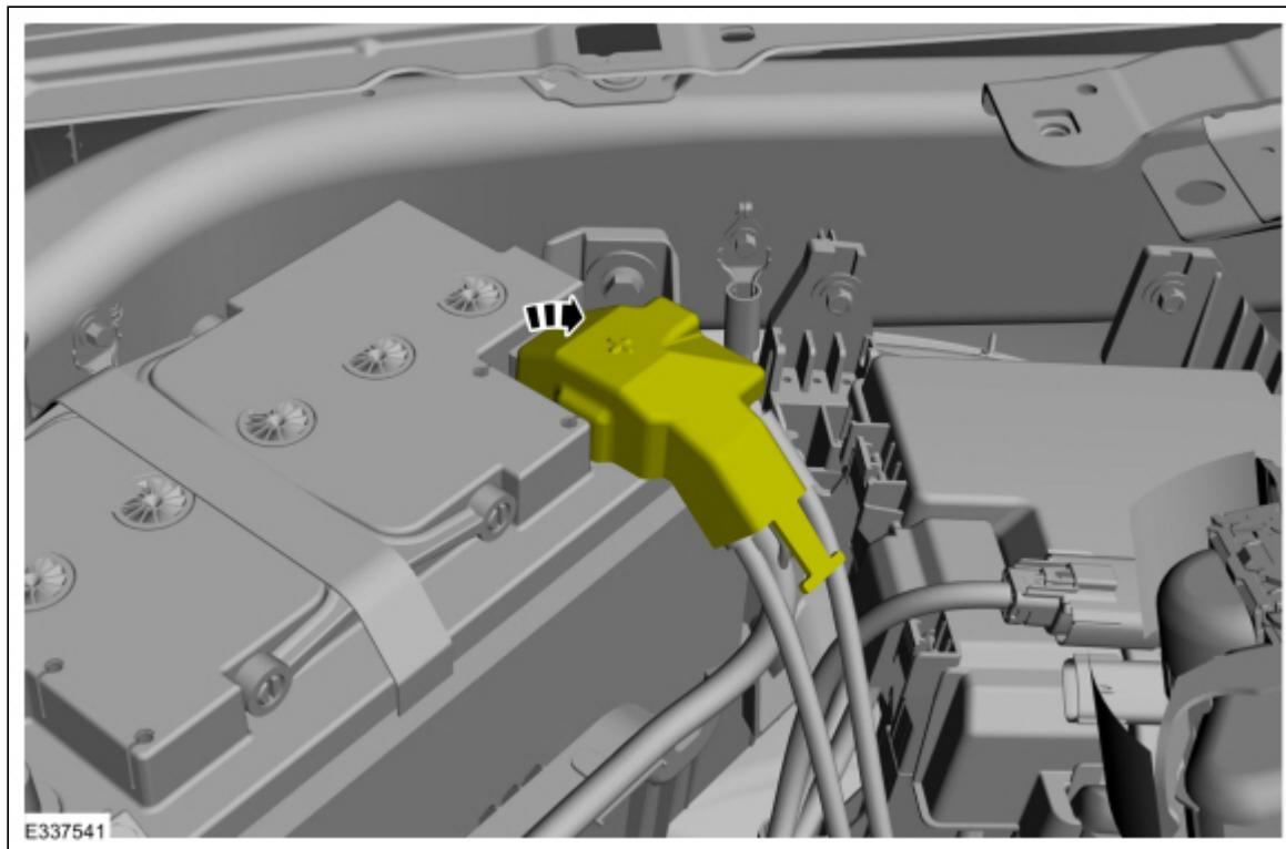
3. Loosen, but do not remove the nut. Position the positive battery cable aside.
