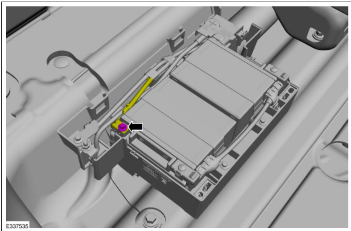
15. Position the positive battery cable terminal cover aside.
