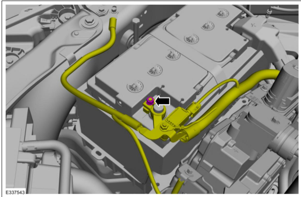
5. Position the positive battery cable terminal cover aside.
