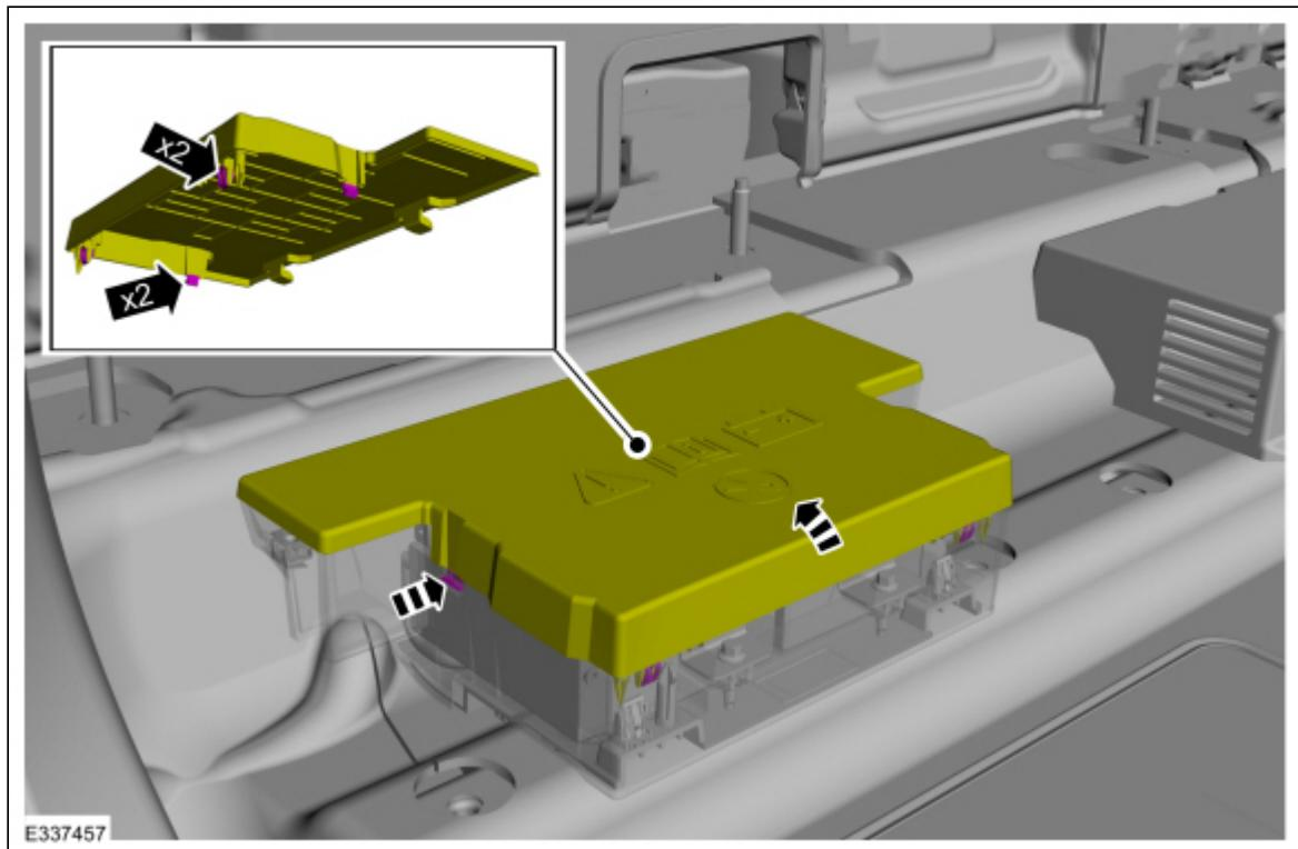
14. **NOTICE:** Make sure the positive battery terminal cover is in position while removing the negative battery cable clamp to prevent damage from a short to the positive terminal.
