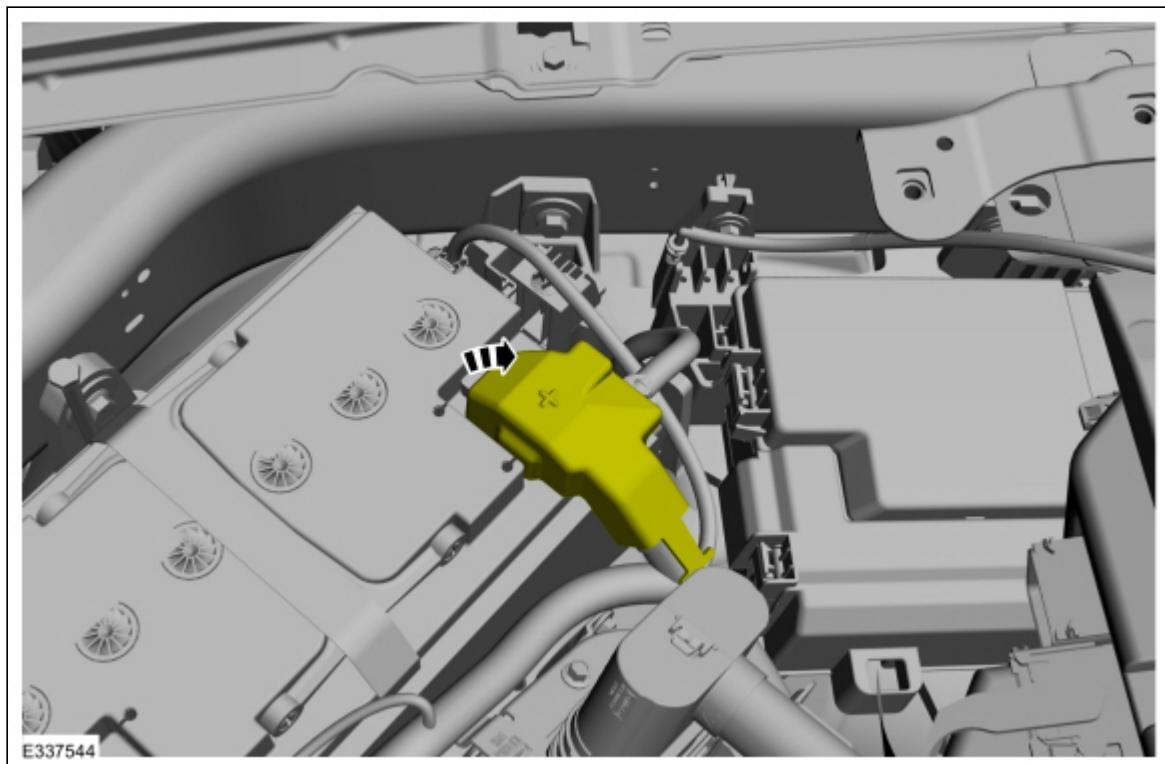
6. Loosen, but do not remove the nut. Position the positive battery cable aside.
