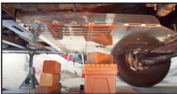
5. Fitment: install plate loosely to and adjust brackets until skid is sitting as high as possible without getting too close to any exhaust components.
