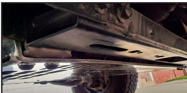
6. Note that a gap in the rear of the skid plate and rear crossmember is normal and good to prevent contact with exhaust components.
