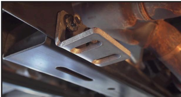
4. Install all four skid plate mounting brackets (two front, two rear). Reuse factory nuts but do not tighten yet.
