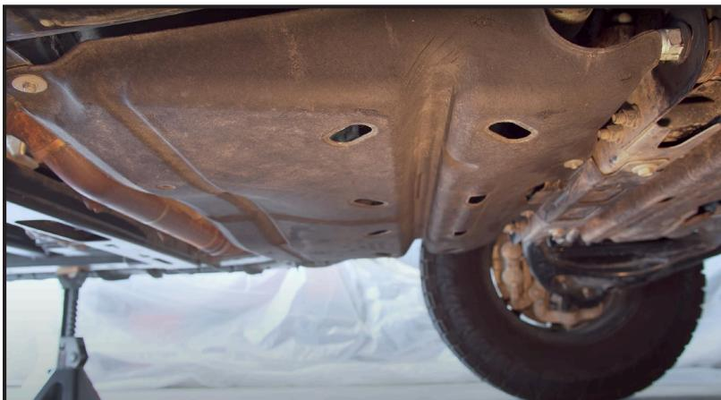
1. Remove factory felt liner. There are four 8mm bolts and two brackets (driver and passenger side) held on with 13mm bolts.
